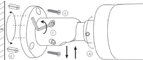
1. Loosen a bit the five hex head studs on the bracket via "L" Allen wrench, for easy installation.
